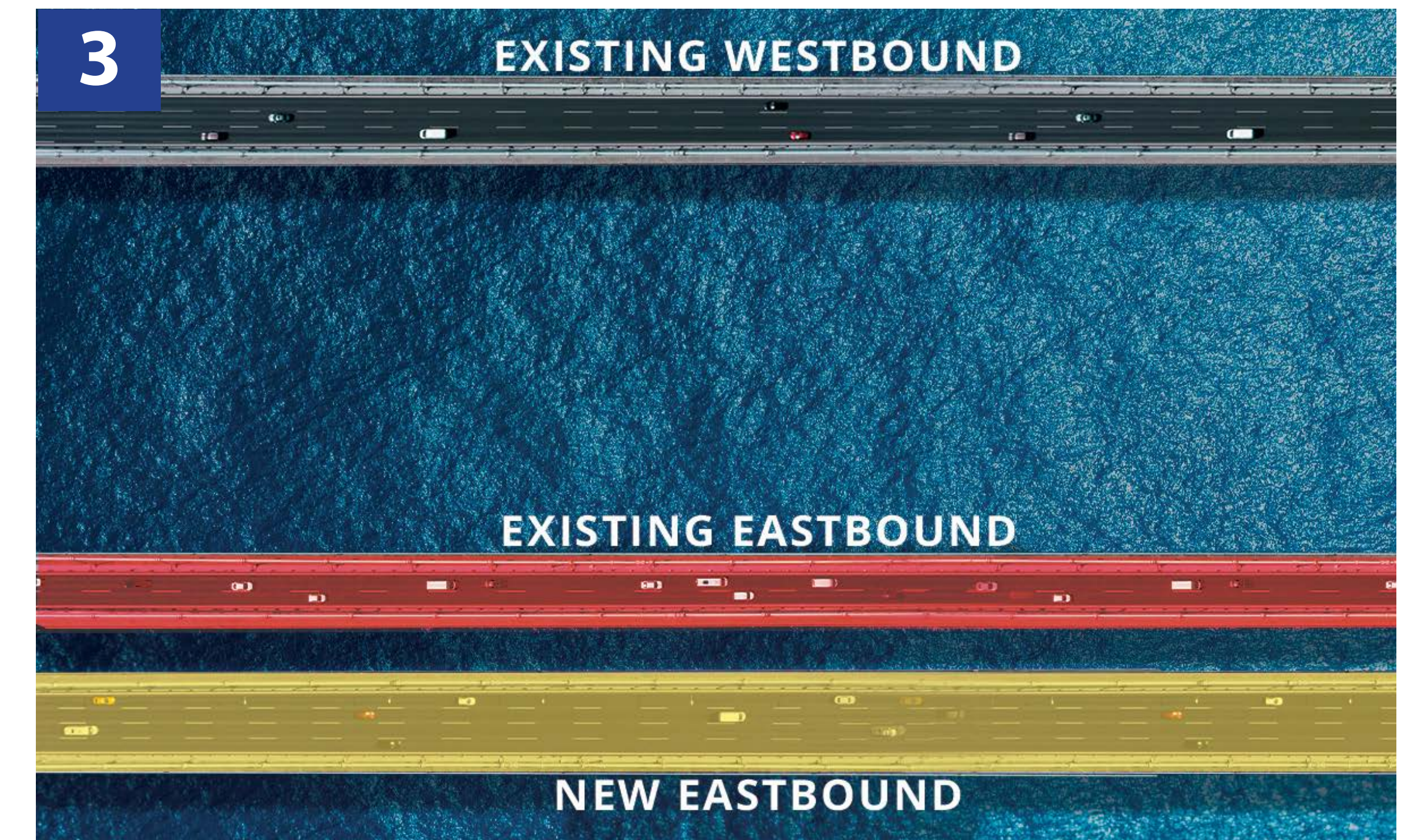
Removal of the existing eastbound span (red) would follow.
