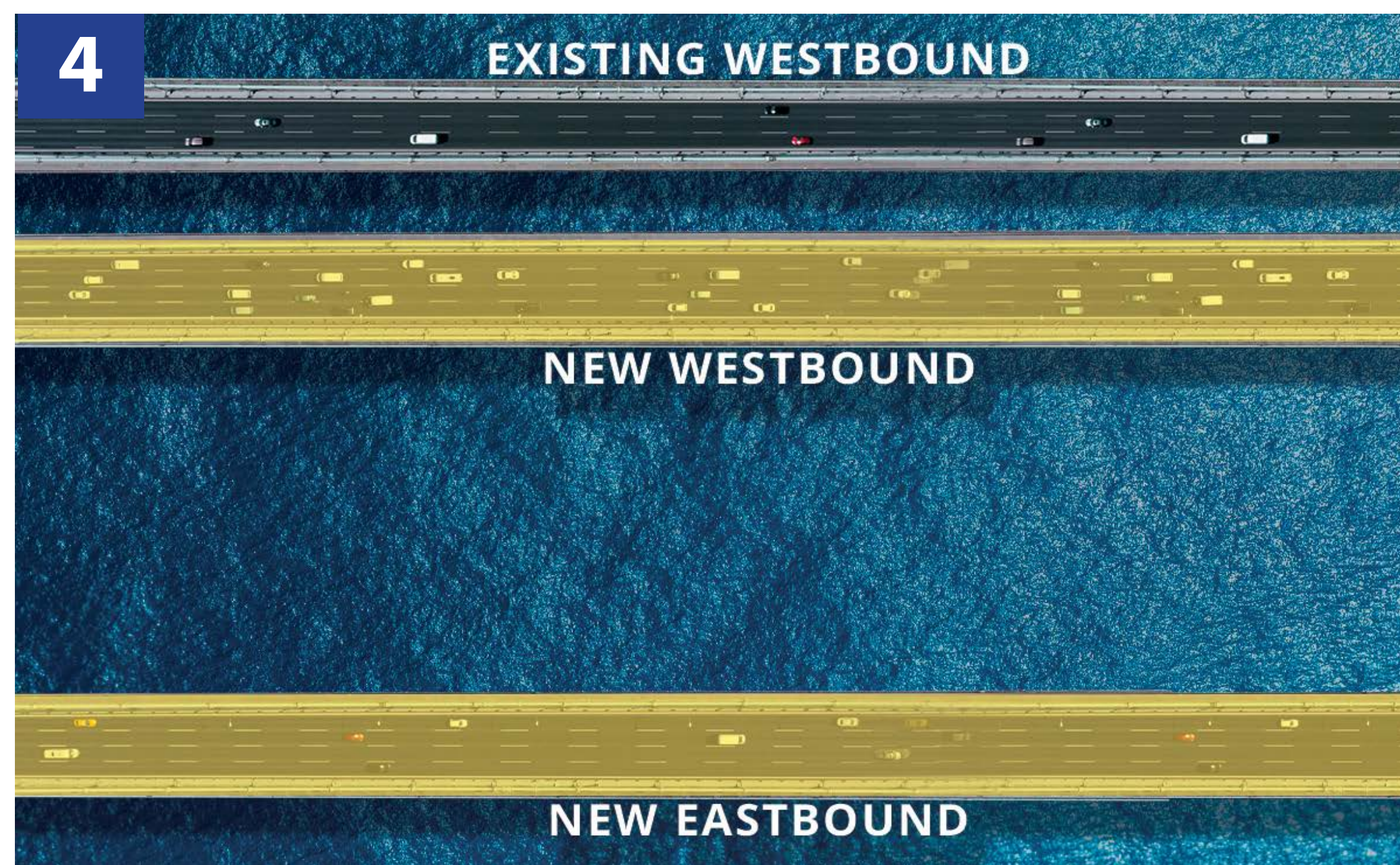
A new westbound span (yellow) would then be constructed between the existing bridge spans.
